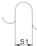
Detail B (Mounting Hole)
