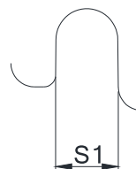
Detail B (Mounting Hole)
